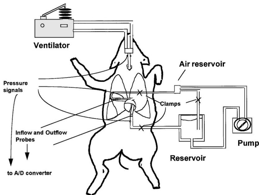
Fig. 1. Experimental setup for constant flow perfusion of pig lungs in situ. Details are explained in text. A/D, analog-to-digital.
