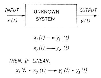
Fig. 1. Input-output relationships for a general communication system. If the system is linear, then superposition of input signals gives rise to superposition of output signals.
