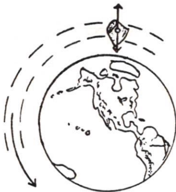
Figure 1. The orbital rate and altitude of a satellite establish a centrifugal field which is equal and oriented 180^\circ to the local gravity field. If these two forces on the satellite are unequal, it will move to an orbit where they become equal.
