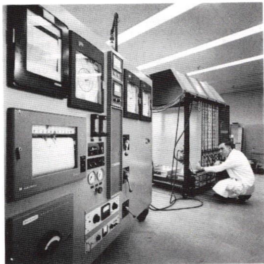
Figure 5. Face view of two-man capacity algal photosynthetic exchanger. Process console at left; illumination console at right.
