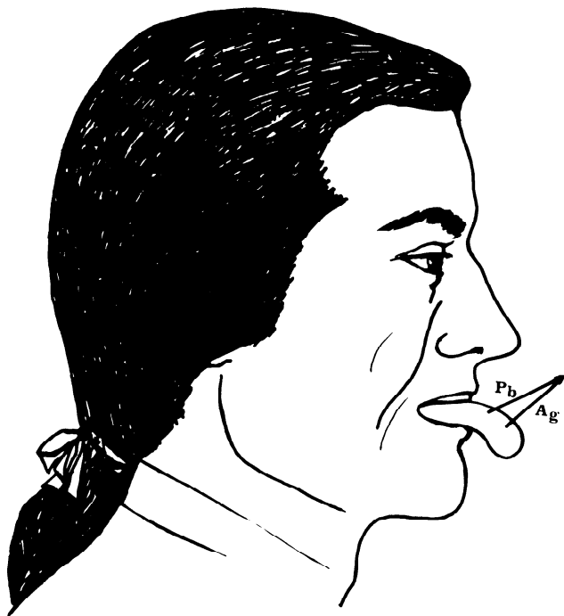
Figure 3-2. The Sulzer experiment which anticipated Volta's discovery of the electrochemical cell. When dissimilar metals were in contact with the tongue, a bitter taste was perceived; either metal alone, or both metals unjoined and on the tongue produced no sensation. (Author's sketch).
