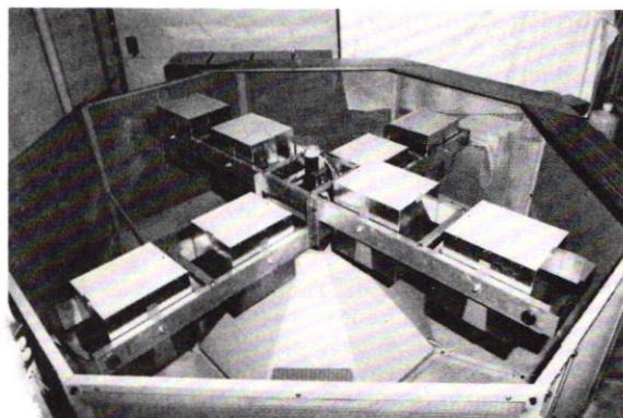
Fig. 1. 1.3m radius centrifuge for animal.
